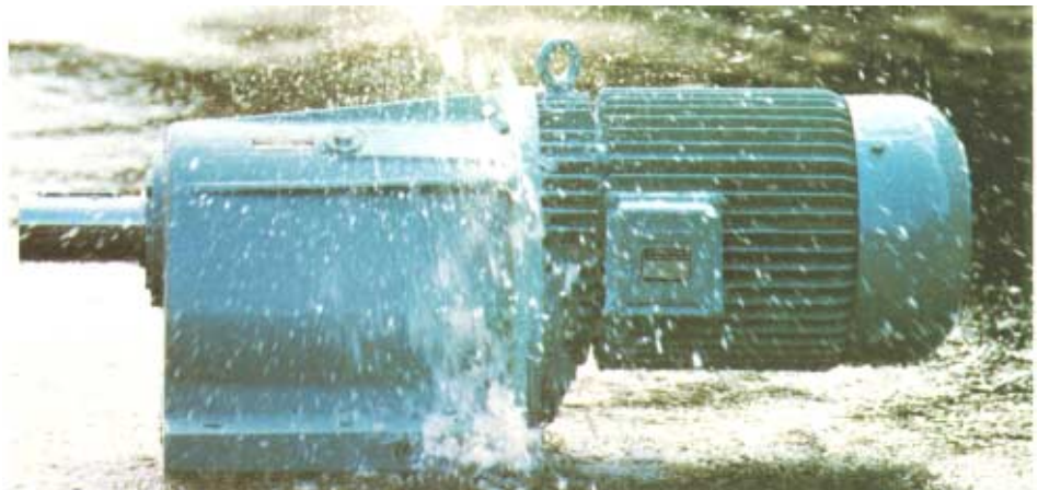
Fig. 8.2.3 Effect of water during the water jet test IPX5
