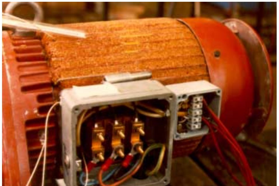
Fig. 15.2.1 Geared motor in a »closed test« with thick layer of dust according to »Practice B« in IEC 61241 and according to North American testing conditions specified by UL and CSA
