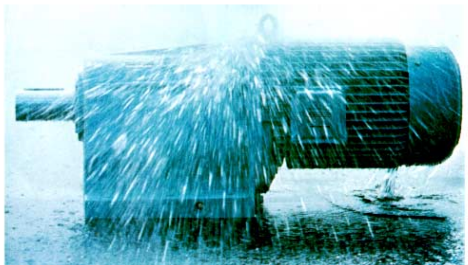
Fig. 9.2.2 Effect of water jet during test for IPX6
