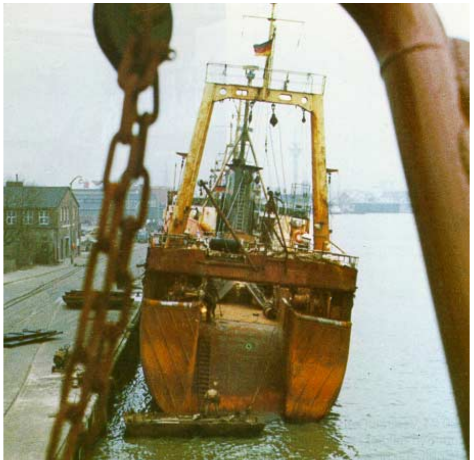
Fig. 26.21 Fishing vessel after several months at sea, showing considerable rust formation.
