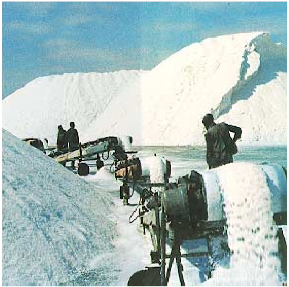
Fig. 14.2.2 Conveyor line made up of mobile belt conveyors with drum motors for salt extraction in a tropical region
