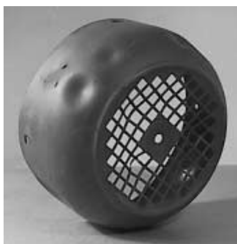
Fig. 20.2 Unreinforced fan cowl (1.0 mm) after the impact test
