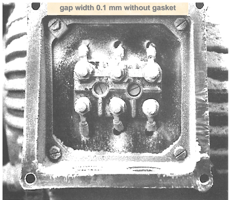
Fig. 11.1.5 Test result with a gap width of 0.1 mm Testing time: approx. 20 minutes
