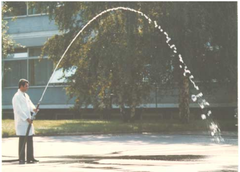
Fig. 8.2.2 Test arrangement for the degree of water protection IP X5 "Water jet"
