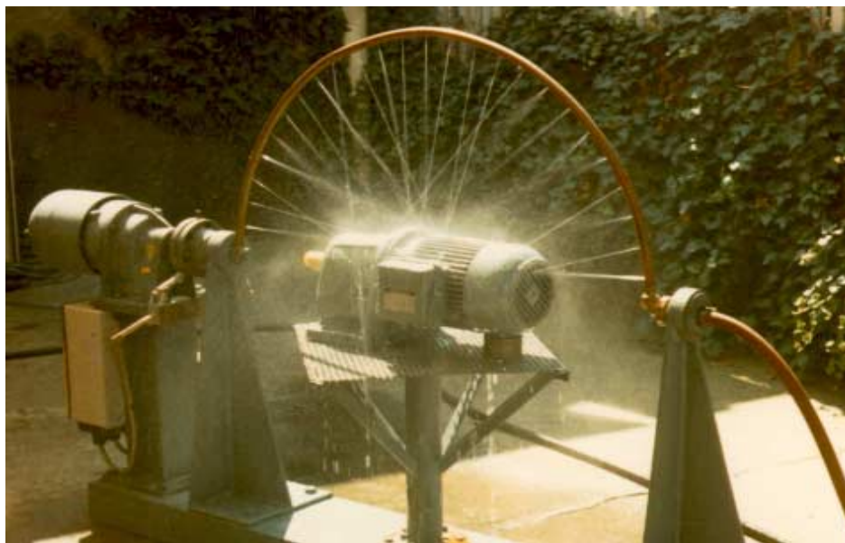
Fig. 8.1.1.2 Oscillating tube for testing the degree of protection against »water spray«
