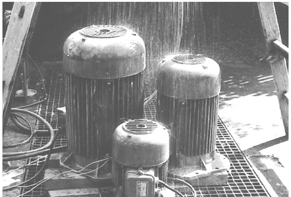
Fig. 23.1 Long-term exposure of geared motors to rain to test fitness for outdoor installation
