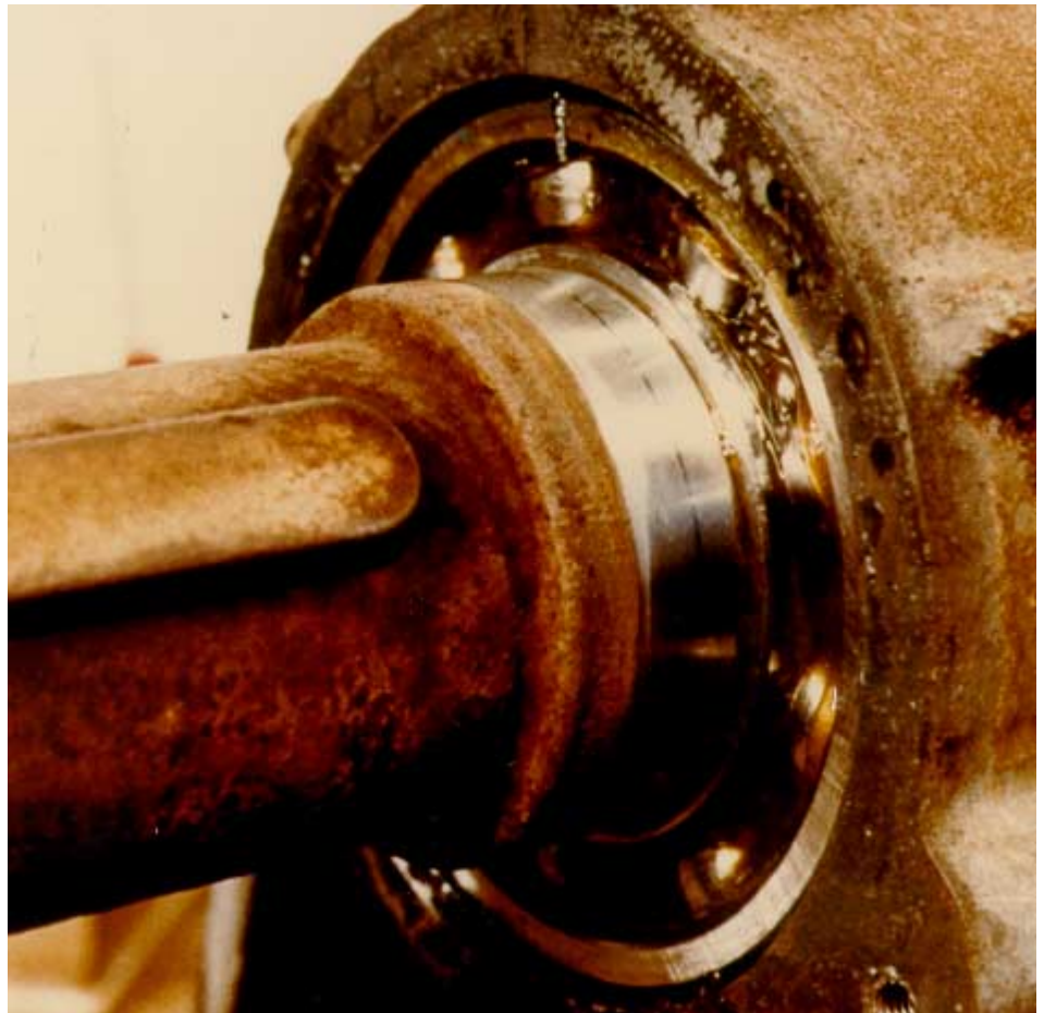
Fig. 26.6 Output shaft of the geared motor in Fig. 26.4. Considerable rusting is visible on the parts exposed to continuous rain for one year, but the perfect condition of the bearing (bearing flange and shaft seal have been removed).
