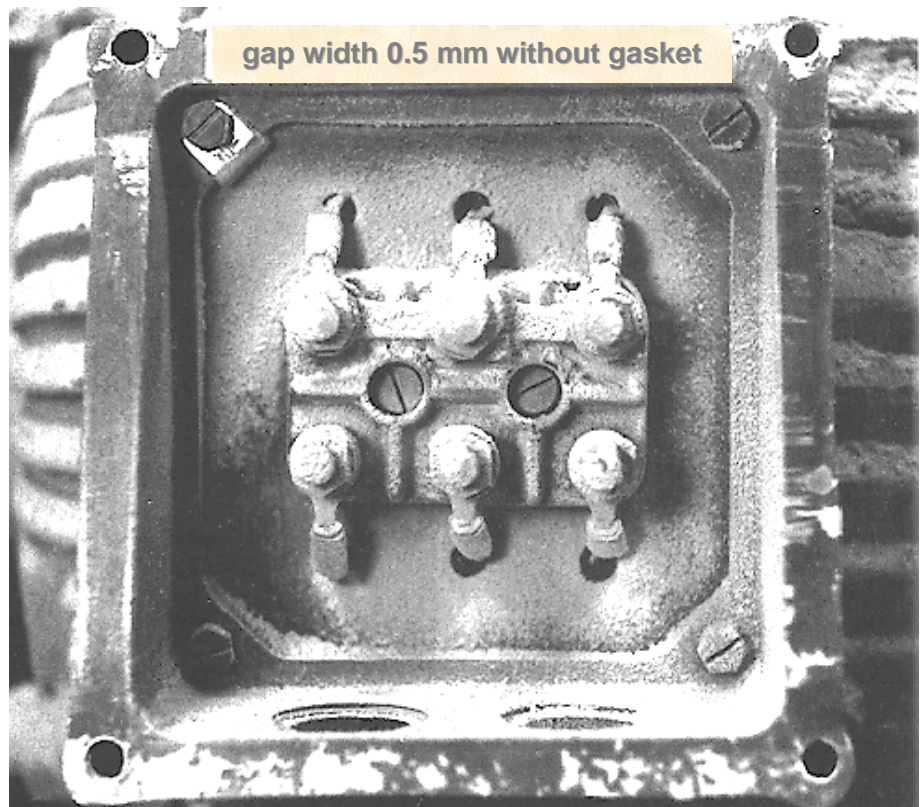
Fig. 11.1.6 Test result with a gap width of 0.5 mm Testing time: approx. 10 minutes
