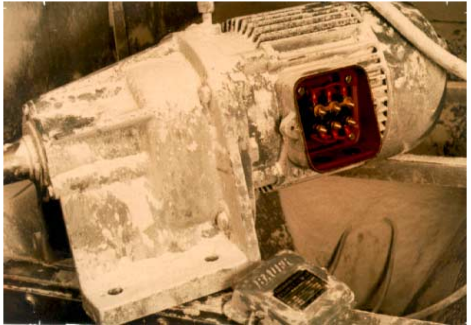
Fig. 10.2.1 Three-phase geared motor after a standard dust test. Terminal box sealed with greased cord. Result: no dust ingress.
