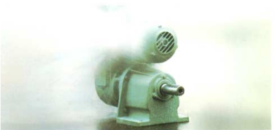
Fig. 8.2.4 Effect of water during the water jet test IP X6 »Powerful water jets«
