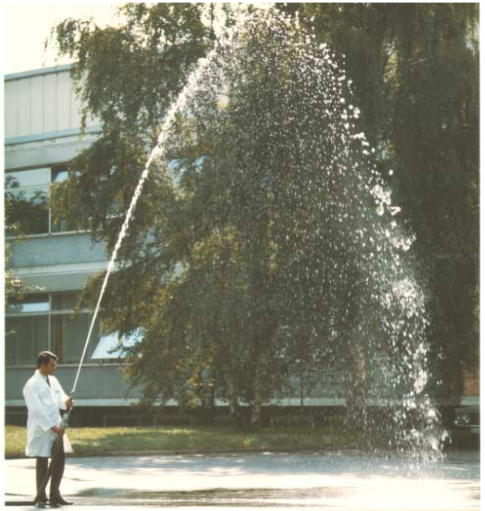
Fig. 9.2.1 Test arrangement for the degree of water protection IPX6 "Powerful water jet"
