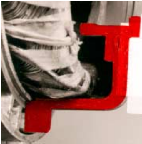
Fig. 13.4.1 Crowding between the end winding and bearing bracket give rise to flashovers in the presence of condensation. A drain hole would not help in these circumstances.
