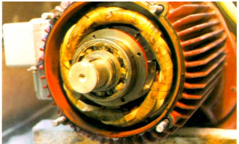
Fig. 10.2.3 Stator of geared motor after standard dust test. Motor interior is completely free of dust.
