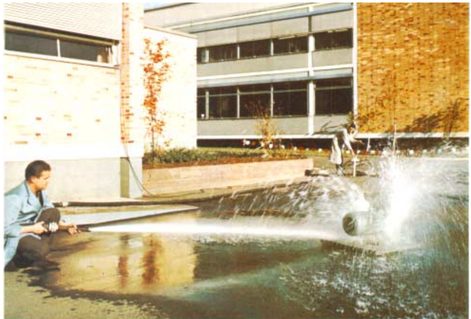
Fig. 9.3.6 Increased severity test of IP66 protected motors with a 25 mm diameter jet and pressure equivalent to an 8 m head
