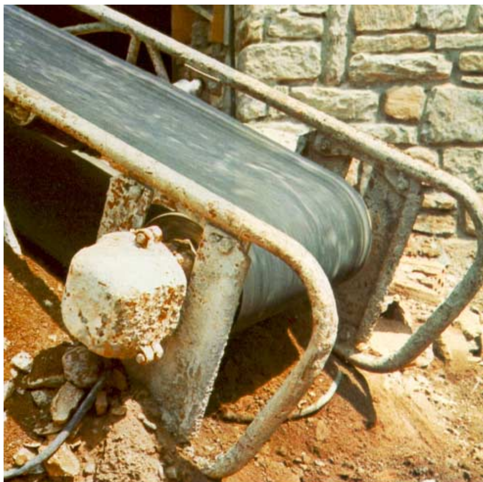
Fig. 19.4.2 Externally affected but fully functioning drum motor on portable belt conveyor under hard construction site conditions
