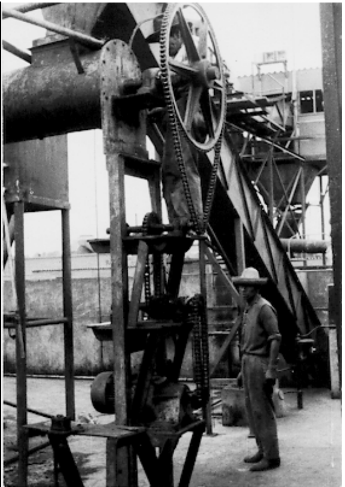
Fig. 12.2.3 Exposed chain transmission on a geared motor in a fish meal factory in Peru
