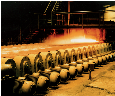
Figure 47.1.1 Shaft-mounted roller-table geared motor on a working roller table
