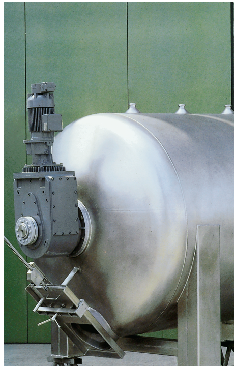
Figure 1.7.5 Shaft-mounted bevel-gear motor on a container.
