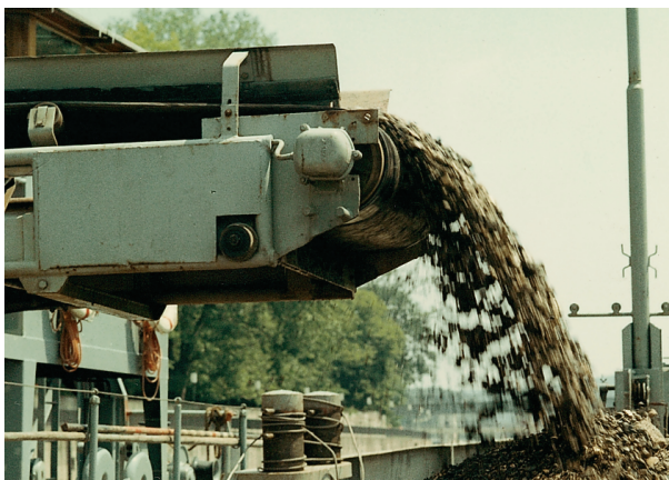
Figure 20.2 Example of application for the S6-60 % duty type: Drum motor for removing intermittently extracted excavation materials from a dredger
