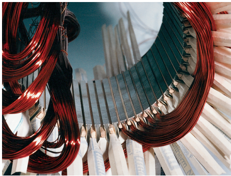
Figure 43.0.1 Manual formation of two separate windings on a pole-changing motor
