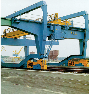
Figure 46.5 Special type DL AC induction motors on the travelling gear of a gantry crane
